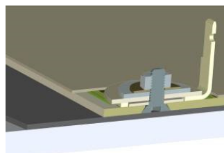
Cross section of contact assembly
